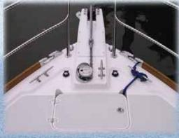
toe rail and molded-in anti-skid surface. On the foredeck, a standard rope/chain windlass is provided for easy anchor management and a large deck well is located aft of the chain locker for fender and line storage. Custom stainless steel mooring chocks forward and amidships, stainless steel portlights and highly polished aluminum hatches are beautiful and practical. They will retain their looks for many years to come.
